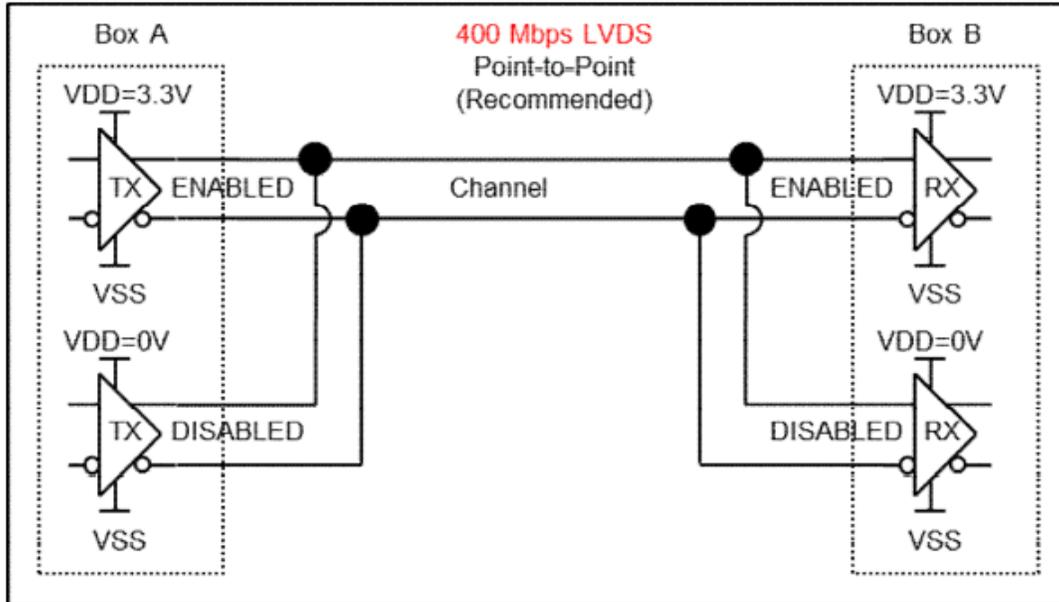
Figure 1: 400Mbps LVDS Redundancy in Point-to-Point Signaling Channels (Recommended)
