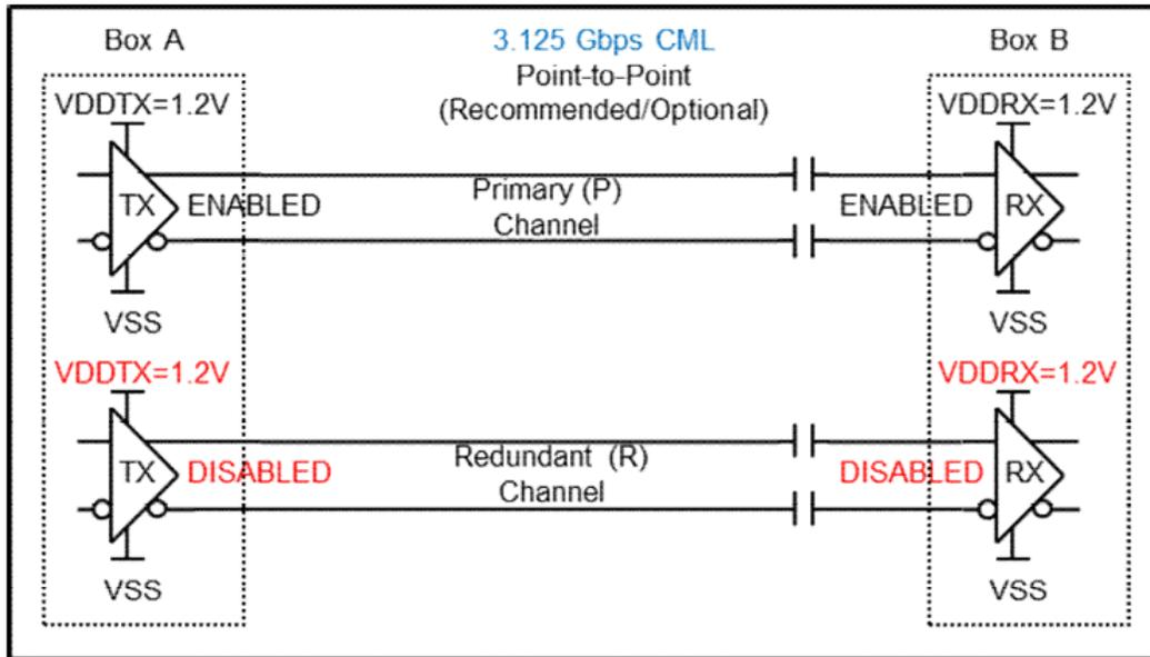
Figure 4: 3.125 Gbps CML Redundancy in Point-to-Point Signaling Channels (Optional).
