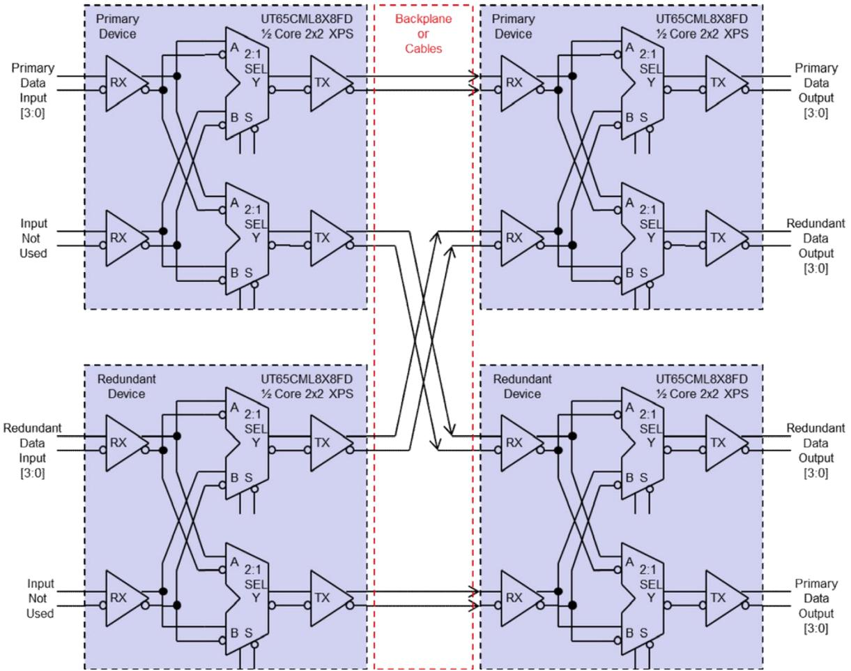
Figure 8: Example: Full Redundancy A-B Cross-Strapping Using Two XPS Devices 3.125 Gbps, 4 Channels Each Data Path, Simplex, Point-to-Point
