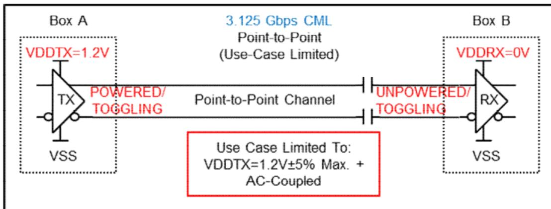
Figure 6: 3.125 Gbps CML Redundancy in Point-to-Point Signaling Channels (Specific Use Case of  $VDDTX=1.2V\pm5\%$  Max.)
