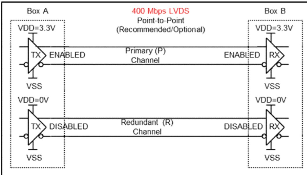
Figure 2: 400Mbps LVDS Redundancy in Point-to-Point Signaling Channels (Optional)
