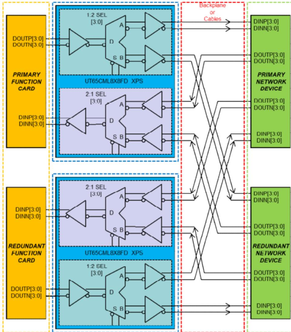
Figure 7: Example: Full Redundancy A-B Cross-Strapping Using Two XPS Devices 3.125 Gbps, 4 Channels Each Data Path, Full Duplex
