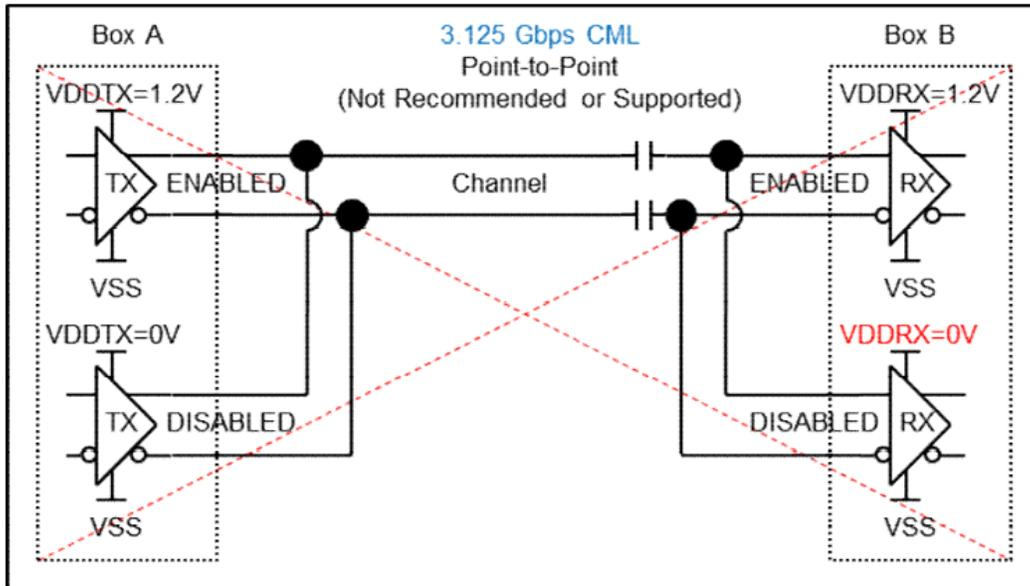
Figure 5: 3.125 Gbps CML Redundancy in Point-to-Point Signaling Channels (Not Recommended or Supported)
