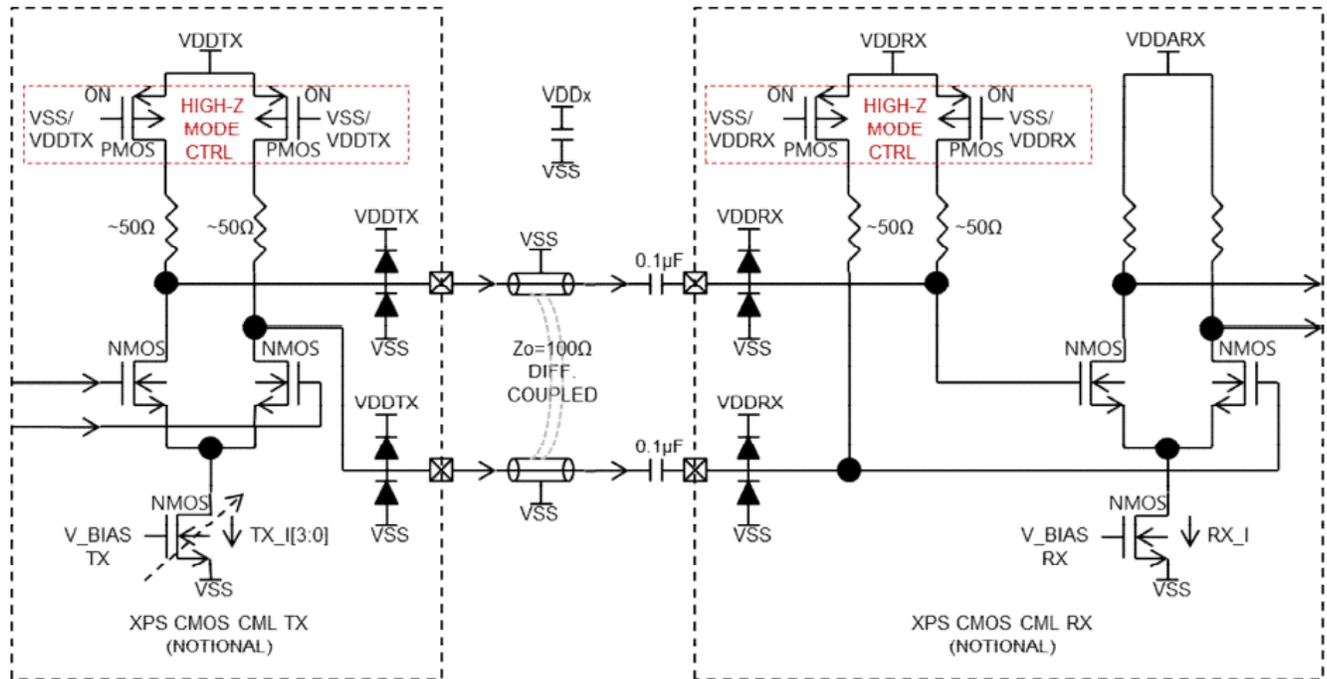
Figure 9: 3.125 Gbps XPS CML TX to RX Point-to-Point Channel – Notional Schematic
