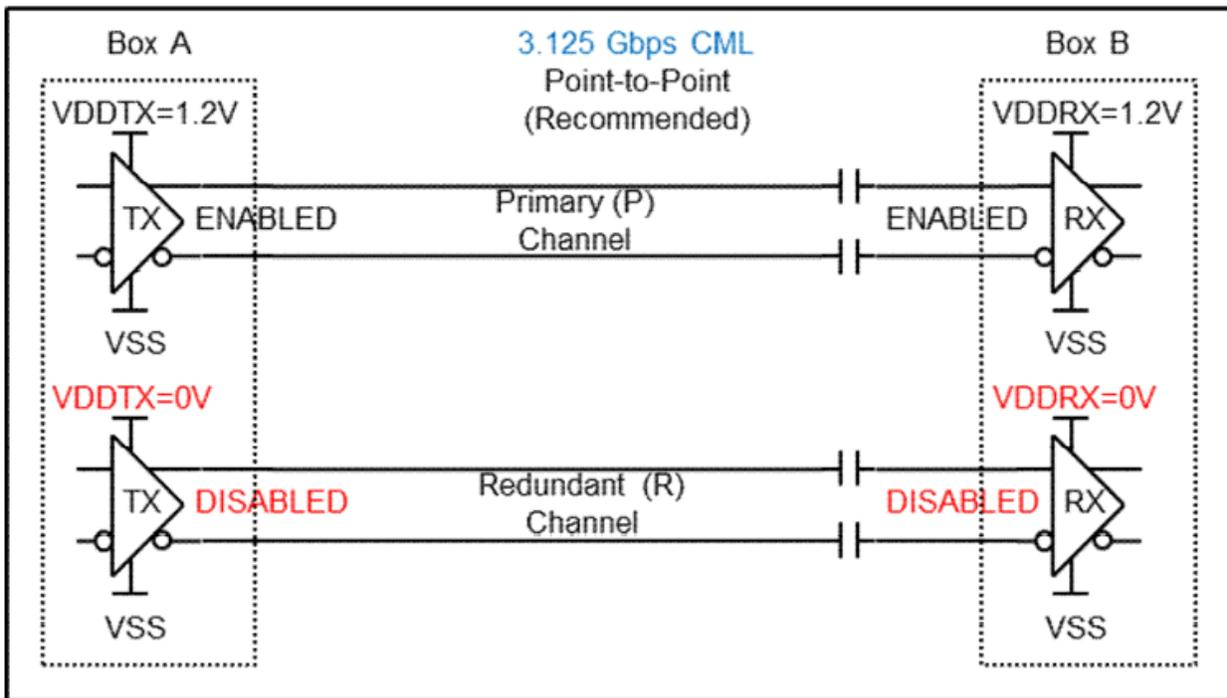
Figure 3: 3.125 Gbps CML Redundancy in Point-to-Point Signaling Channels (**Recommended**).
