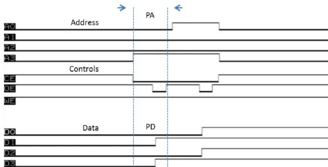
Figure 4: Read Command Sequence Timing Diagram
