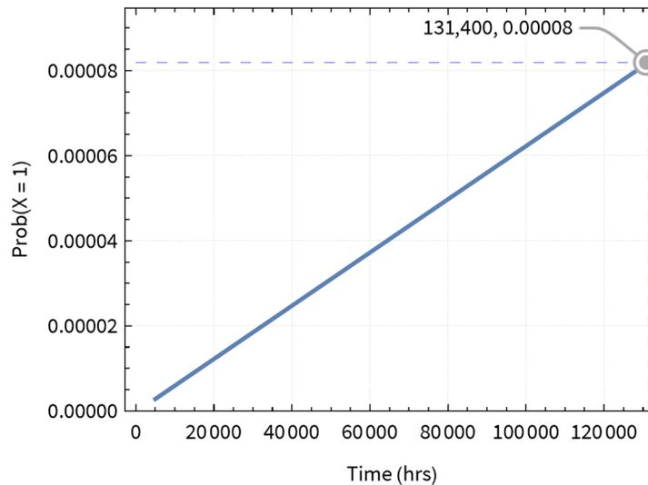
Figure 9: Plot of equation (6) showing probability of 1-bit error in a 48-bit word over time.
