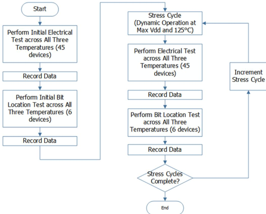
Figure 1: Flow diagram of experiment stress-measure-stress cycles.
