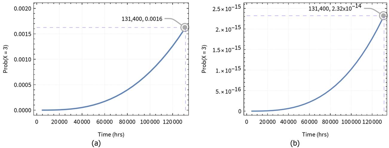
**Figure 14: Plot of probability of 3-bit errors in a 48-bit word over time for (a) Rows 0 and 1 only using equation (7) and (b) all other rows using equation (8).**
