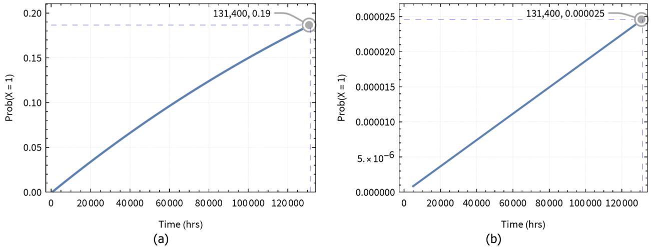
**Figure 12: Plot of probability of 1-bit error in a 48-bit word over time for (a) Rows 0 and 1 only using equation (7) and (b) all other rows using equation (8).**
