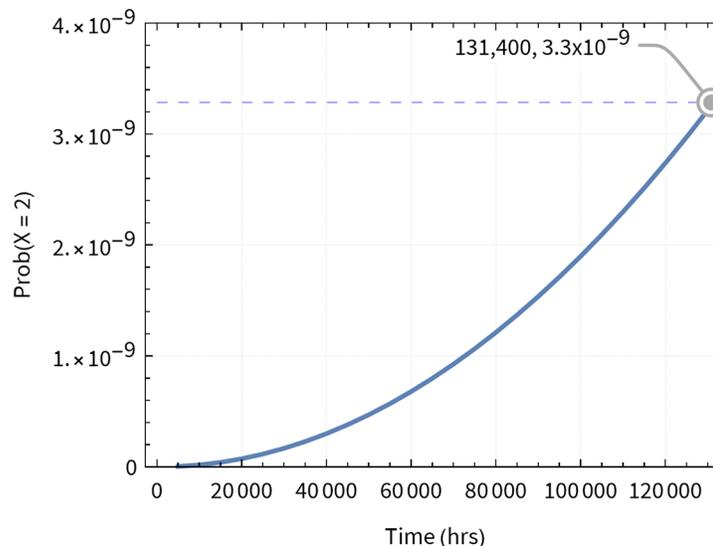
Figure 10: Plot of equation (6) showing probability of 2-bit errors in a 48-bit word over time.
