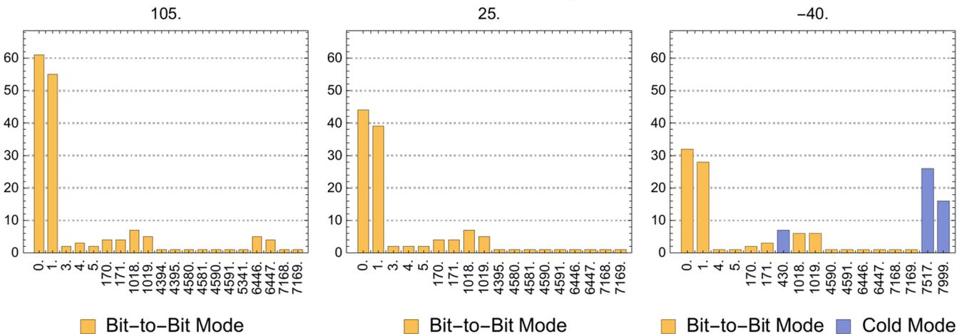
Figure 6: Graphs showing unique bit errors per row for both the Bit-to-Bit and Cold modes for each of the test temperature from the bit location testing.
