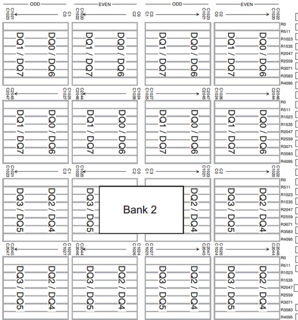
Figure 7: Illustration of DQ relationship in the memory architecture.
