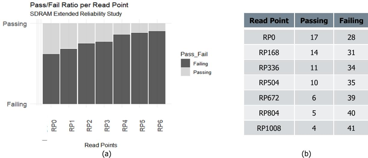
**Figure 2: Trend results from production testing showing increasing bit errors at the end of each stress cycle. (a) Mosaic plot showing passing and failing trend. (b) Numerical account of passing and failing.**
