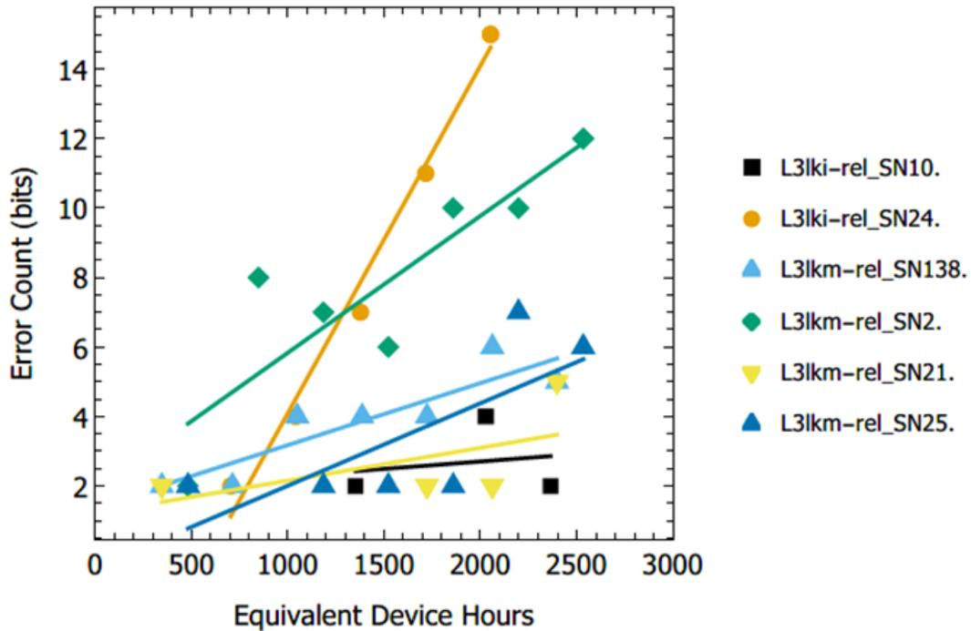
**Figure 8: Plot of bit errors and regression models for the each of the devices. Data is from the 105°C bit location testing.**
