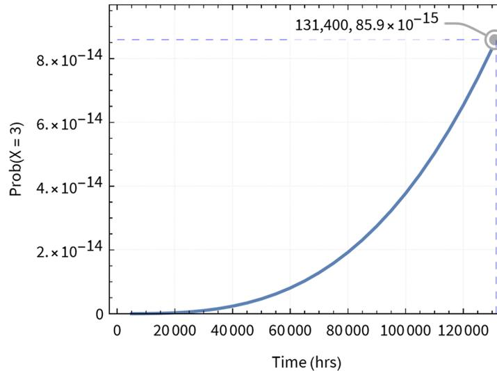
Figure 11: Plot of equation (6) showing probability of 3-bit errors in a 48-bit word over time.
