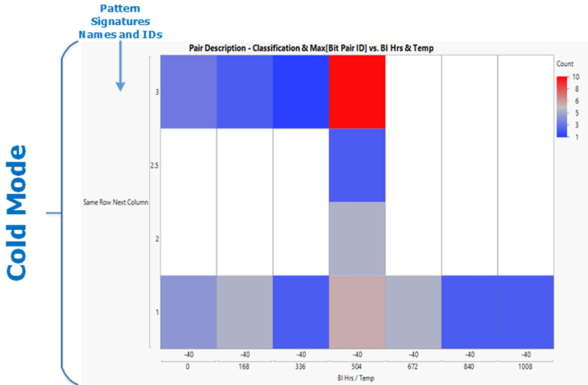
Figure 5: Graph showing Cold Mode bit errors for each stress cycle as a function of temperature. Numbers in the y-axis are row numbers associated with the pattern signature.
