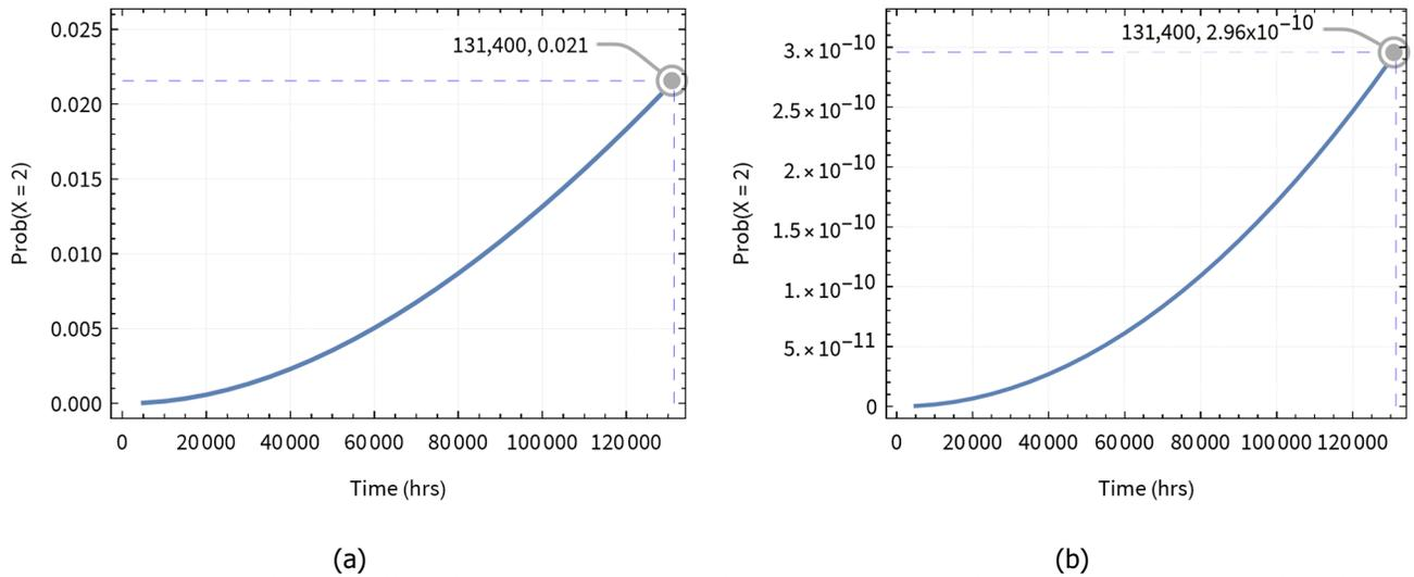
**Figure 13: Plot of probability of 2-bit errors in a 48-bit word over time for (a) Rows 0 and 1 only using equation (7) and (b) all other rows using equation (8).**
