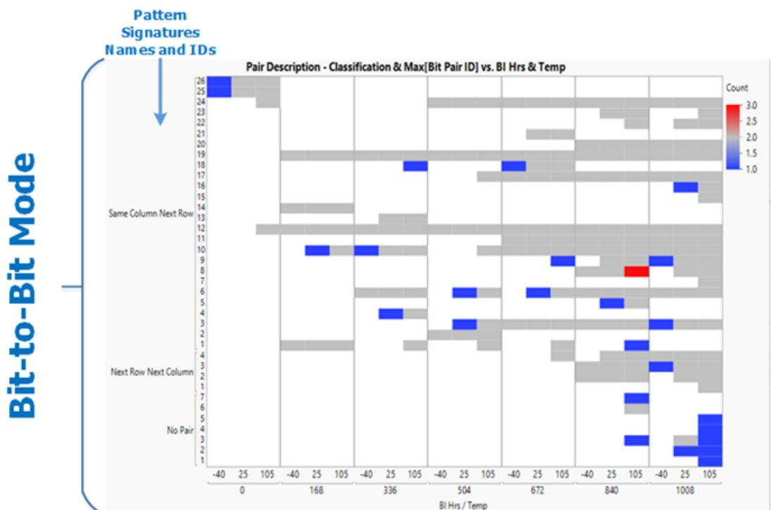
**Figure 3: Graph showing Bit-to-Bit Mode bit errors for each stress cycle as a function of temperature. Numbers in the y-axis are row numbers associated with the pattern signature.**
