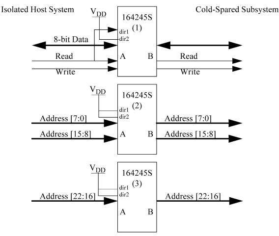
Figure 3. UT54ACS16425S Cold-Sparing Control
